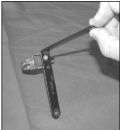
25. Secure the vacuum switching valve to the provided "L" bracket using the provided hardware as shown.
