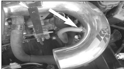
37. Reconnect the EVAP OBD canister closed valve vent hose to the vent on the Typhoon intake tube as shown.
