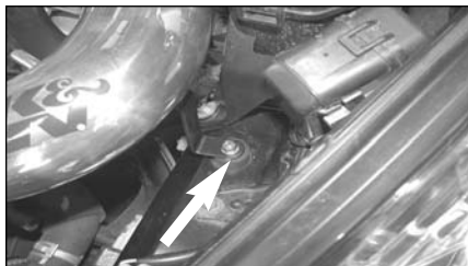
36. Line up the "Z" bracket with the rubber mounted stud and secure it with the provided hardware as shown.
