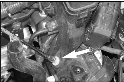
29. Loosen and remove the stock nut on the relay and fuse box support bracket as shown.
