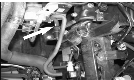
33. Reconnect the vent hose removed in step 23 to the EVAP OBD canister closed valve as shown.
