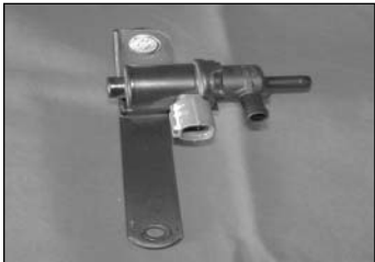
24. Secure the EVAP OBD canister closed valve to the provided angle bracket using the provided hardware as shown.
