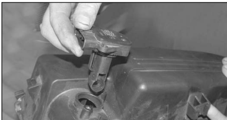
20. Remove the mass air sensor from the air cleaner assembly as shown.
