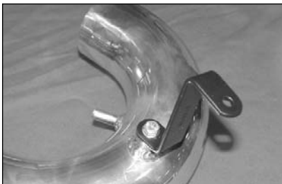
26. Secure the "Z" bracket to the threaded boss on the Typhoon intake tube using the provided hardware as shown. NOTE: Before installing the "Z" bracket, inspect the inside of the tube for any debris, then clean the inside out with water and a towel. Inspect the tube one more time before proceeding to the next step.
